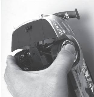
In order to install the electronics, the body must be detached. Turn the car over, and hold the rear wheels with your hand.
