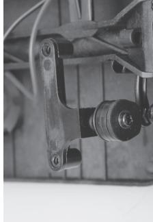
As shown in the upper and lower photos on the left, lift up the servo saver stay and rotate it 180 degrees to where it is upside down.
