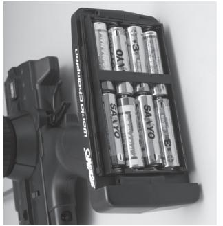
Place eight AAA-size batteries into the transmitter. Make sure that the polarity(+/-) is correct when putting in the batteries.
