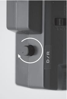
The knob located on the upper left panel is D/R (Dual Rate, or the maximum amount of steering angle). Once all of the electronics have been installed, use this knob to adjust the car's maximum amount of steering angle.
