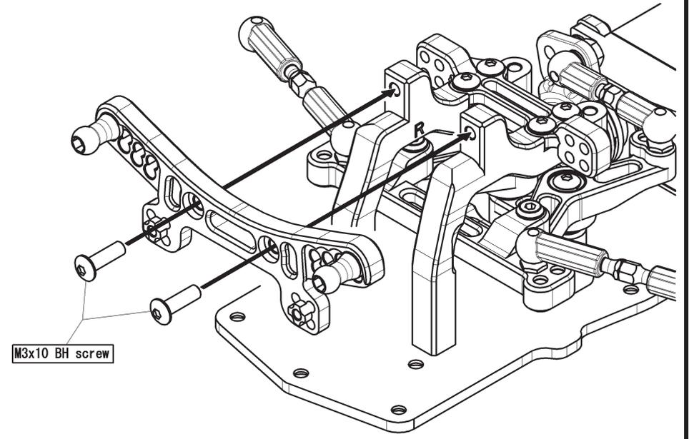
**Installing on rear shock tower**
