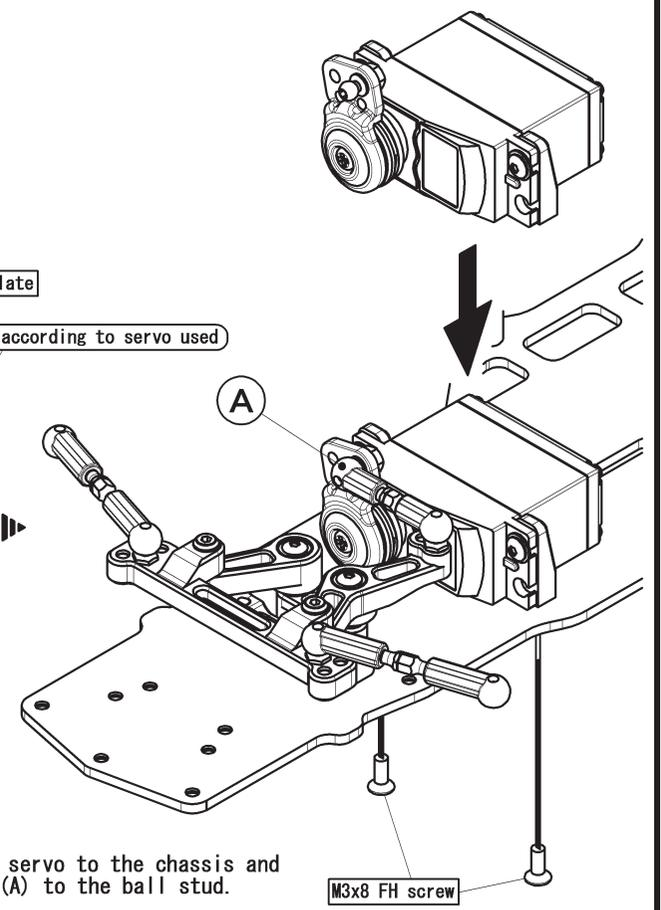
Install the servo to the chassis and attach rod (A) to the ball stud.
