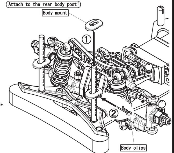
Slide the body mounts onto the body posts to the desired position. Line up the hole on the body mount and body post, and insert a body clip to secure. (Repeat for all body posts.)
