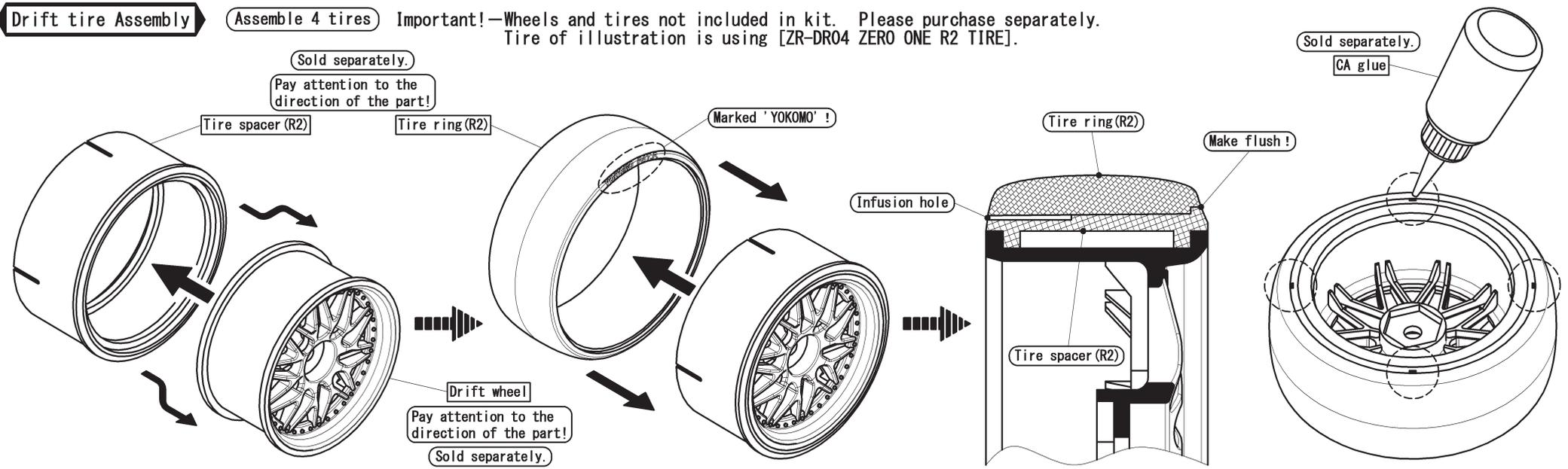
Install the tire spacer onto the wheel.
