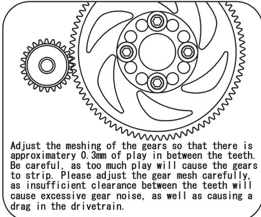
Adjust the meshing of the gears so that there is approximately 0.3mm of play in between the teeth. Be careful, as too much play will cause the gears to strip. Please adjust the gear mesh carefully, as insufficient clearance between the teeth will cause excessive gear noise, as well as causing a drag in the drivetrain.
