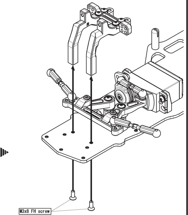
**Installing on front shock tower**
