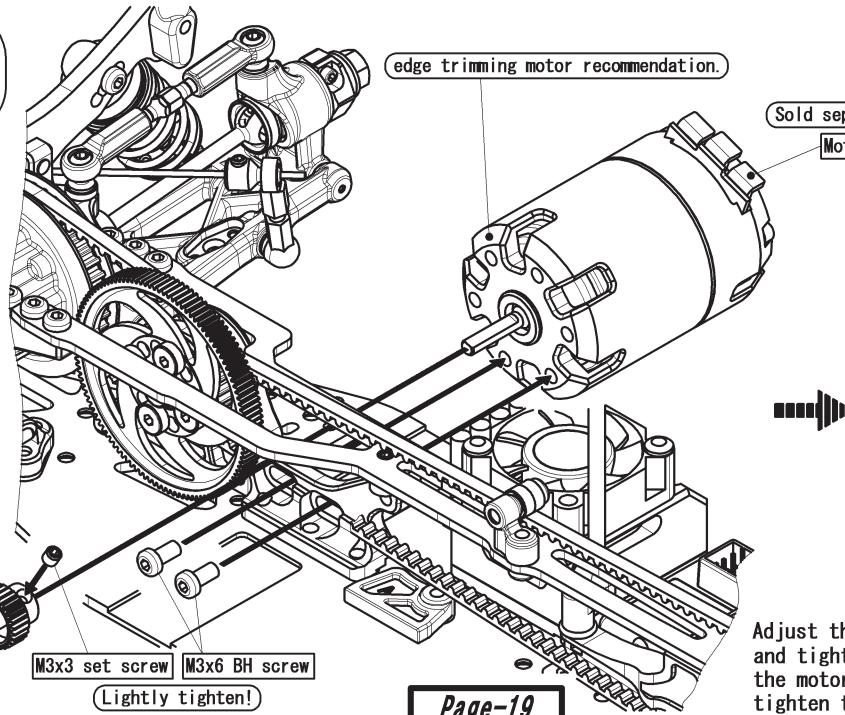
Adjust the pinion so that it lines up with the spur gear and tighten the set screw to secure the pinion. Adjust the motor position so that the gears mesh correctly and tighten the two button head screws to secure the motor.
