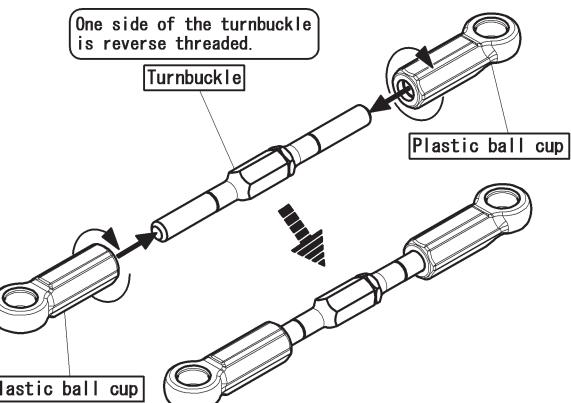
Assemble the tie-rod by attaching a plastic ball cup to both ends of the turnbuckle.
