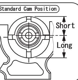
To adjust belt tension, slightly loosen the bulkhead cap screws, and reposition the cams as shown in the illustration.
