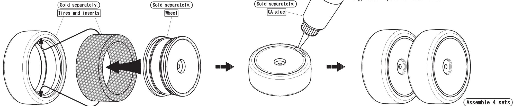
Pull the sidewall of the tire slightly away from the rim and apply CA(Cyanoacrylate) glue in between the tire bead and rim. Make sure that the bead settles onto the rim properly after each application. Slowly work your way around the tire. Allow glue to dry, then repeat on other side.
