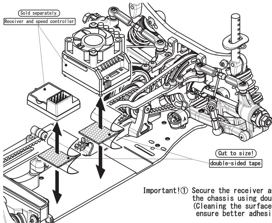
**Important!①** Secure the receiver and speed controller to the chassis using double-sided tape.
