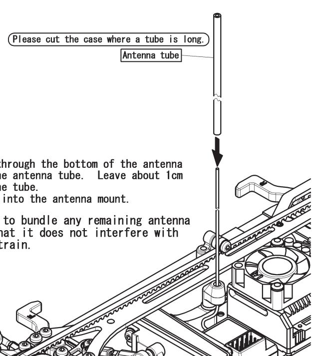
Slide the antenna wire through the bottom of the antenna mount and insert into the antenna tube. Leave about 1cm of wire at the top of the tube.
