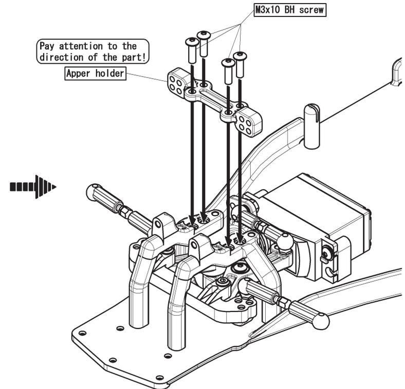
**Installing on front shock tower**
