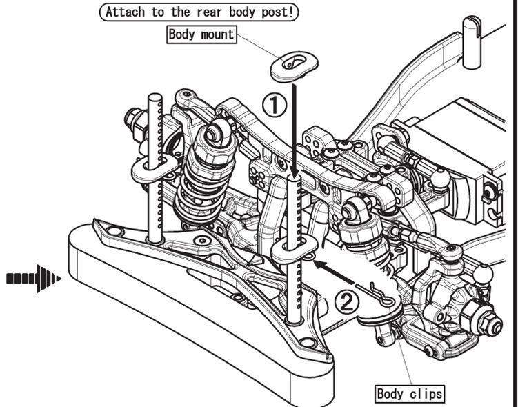
Slide the body mounts onto the body posts to the desired position. Line up the hole on the body mount and body post, and insert a body clip to secure. (Repeat for all body posts.)
