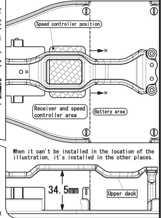
When it can't be installed in the location of the illustration, it's installed in the other places.
