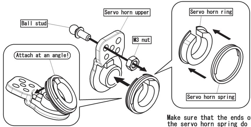
As shown in the illustration, attach the servo horn ring at an angle.
