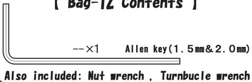
All of the 3mm set screws included in this kit are allen head set screws. To tighten, please use a 2.0mm allen wrench or the 2.0mm allen key included in this kit.
