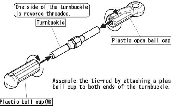
Assemble the tie-rod by attaching a plastic ball cup to both ends of the turnbuckle.
